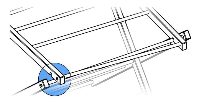
To rectify this, gently rack the latches (bending it in the direction opposite its current "twist") until both bars look parallel and both latches engage fully:
