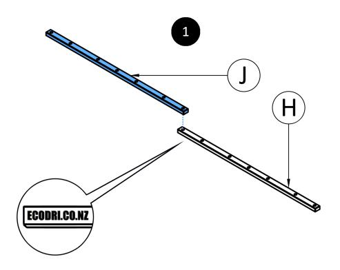
The "H" bar is branded. Place the brand on the side where both bars meet.
