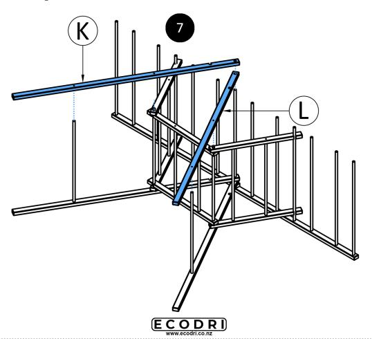
It is almost the end! Take the remaining bars and place them on top, aligning all dowels with the holes. Remember : work from one end to the other.
