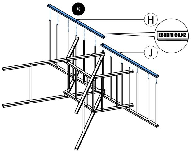
You can now screw the dryer together. Start with one side. One person can hold on to the dowel while the other screws it in. Ensure the screws firmly seat the bar onto the dowels:
