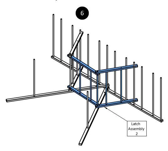
Add two bars on top of these parts, securing "Latch Assembly 1" and "Latch assembly 2" into place:
