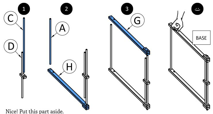
Now we will build the "top". The steps are similar. This time, there are four dowels to fit in. To do so, start fitting the dowel on one end, then work your way through to the other end. If you have someone helping, we recommend having one person bumping the bar into place while the other keeps the rest of the dowels aligned:
